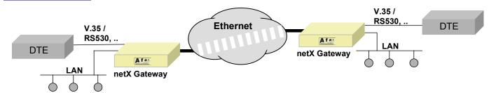
The Afar NetCrossing™ gateway breaks a continuous serial data stream into fixed size packets, adds the Ethernet or IP framing, and sends them over a packet switch network to a remote gateway. At the remote end, the gateway removes the Ethernet or IP framing and reconstructs the original data stream. The gateways regenerate the clocks and keep both ends synchronized with no bit slips.
