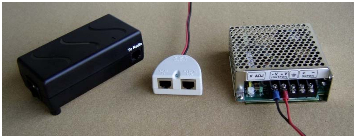
Figure 1.2 – Power Inserter Units and DC/DC Converter
