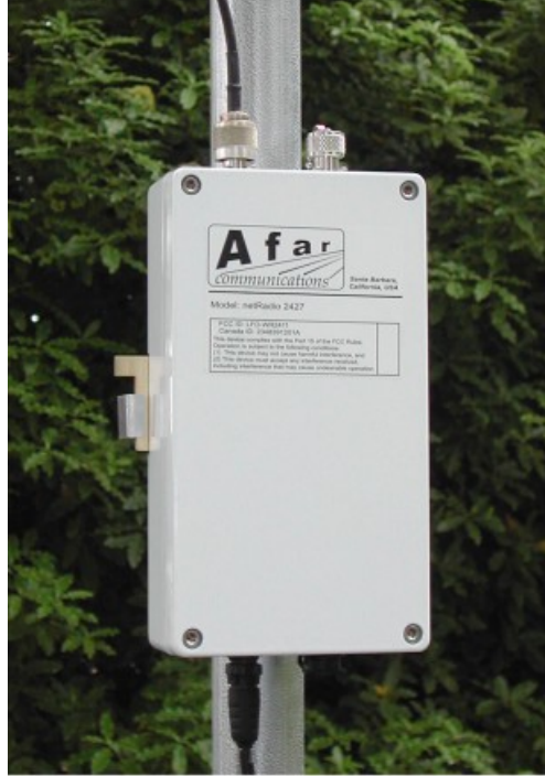
Figure 1.1: Pole Mounted Radio
