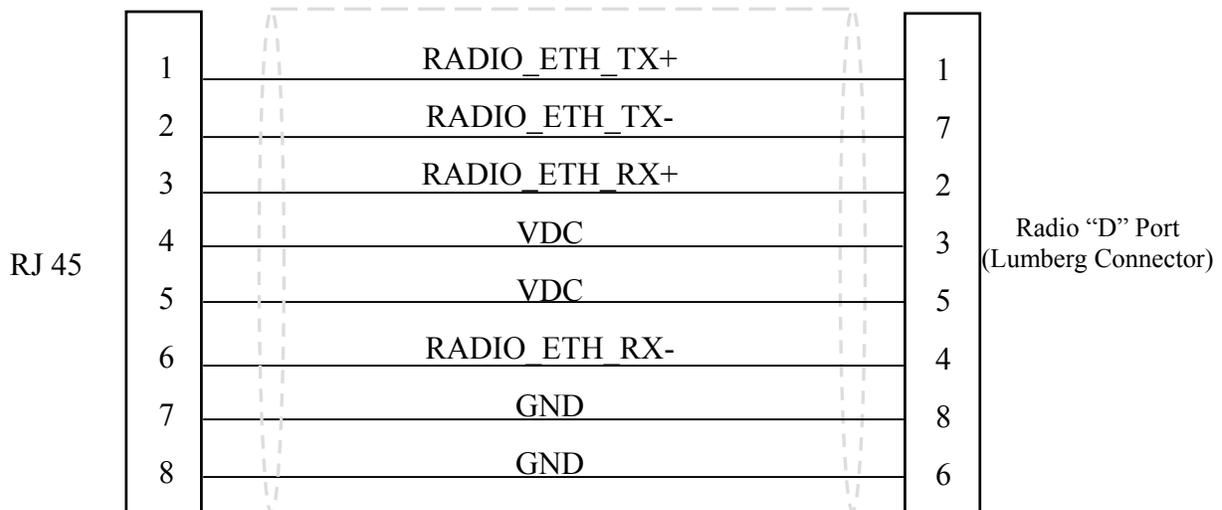
**Figure 1.3 - CAT 5 Outdoor Interconnect cable diagram**
