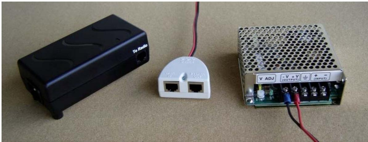
**Figure 1.2 – Power Inserter Units and DC/DC Converter**
