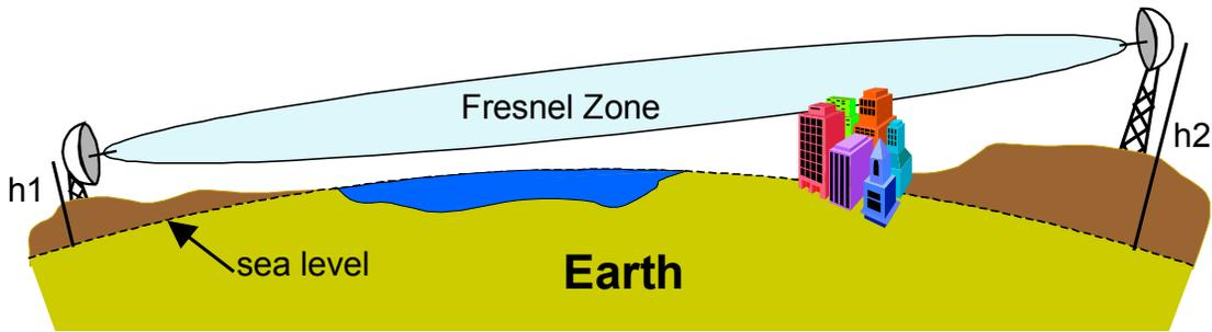
Figure 6.1 – Earth curvature, Fresnel Zone and antenna heights
