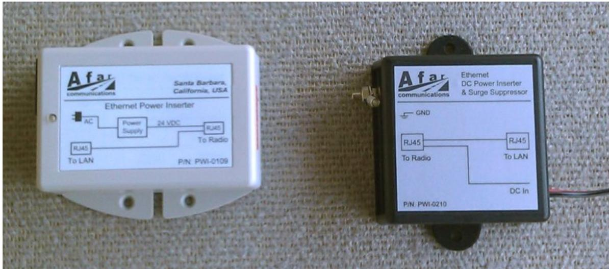
**Figure 1.2 – AC (left) and DC (right) Power Inserter Units**
